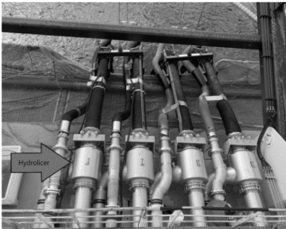
Fish being pumped into the four main lines; arrow shows hydrolicer
